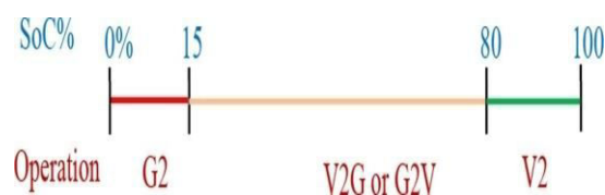
Fig 5.2: Operation modes based on battery SoC%
